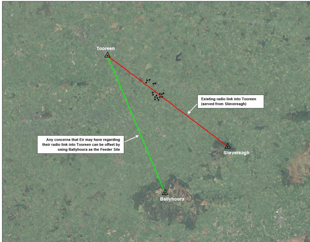
Figure 13. Example of how an alternative feeder-site could be used to mitigate against an obstructing turbine.
